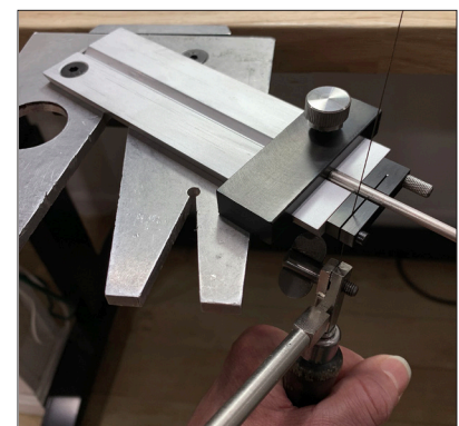
Jig mounted on Jayne Redman® Rotational Bench Pin for hands free use. This is my position for sawing left handed.
