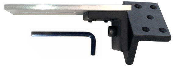
1. Standard Rotational Base rotated with the Aluminum Work Surface attached. To change the angle of rotation, use the large hex wrench to loosen the 3/8" socket head screw attaching the two Universal Mounting Brackets together.
