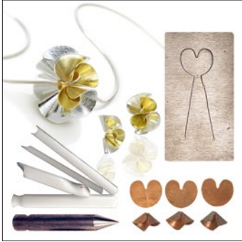
Making Multiples with Blanking Dies
